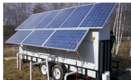
Photo of a solar powered remediation trailer for 1,4 dioxane.
